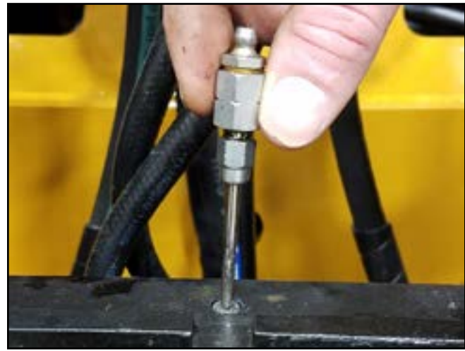
Needle grease tip adapter. This is needed to grease the sideshift.
