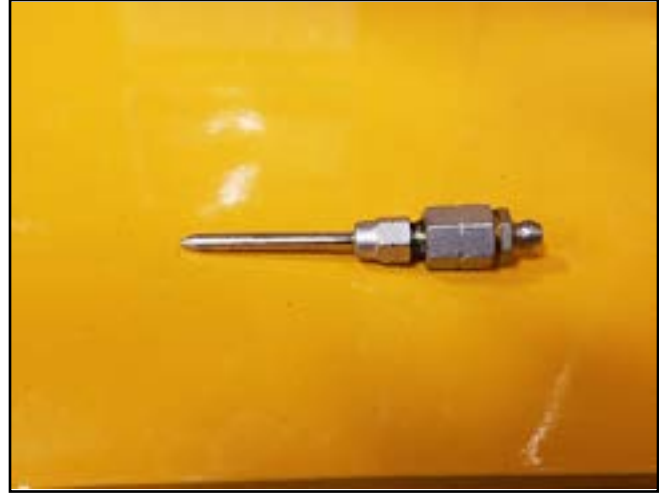
Needle grease tip adapter. This is needed to grease the sideshift.
